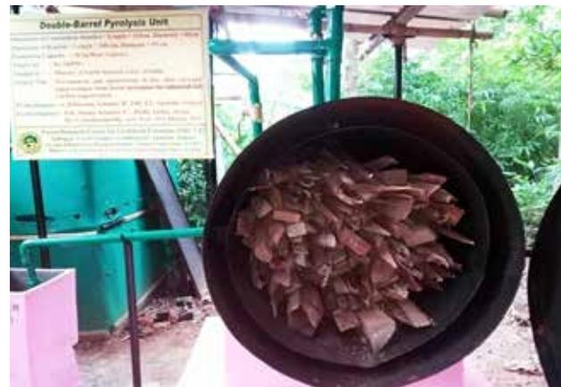
Double-Barrel Pyrolysis System
