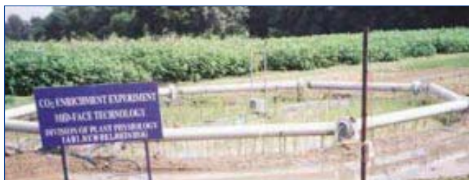
FACE set-up at the Indian Agricultural Research Institute to study the impact of increased CO 2 on crops.
