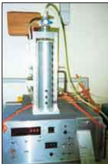
Aerosol size distribution measuring equipment—QCM cascade impactor at one of the Indian laboratories.
