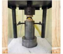
Rotational wood welding machine holders
